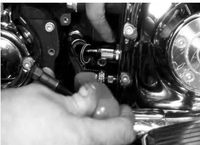
11. With oil, lube both fittings and put male fitting into female and secure with clamshells. Clamshells have small gap, leave gap facing outwards for easy spring removal.
