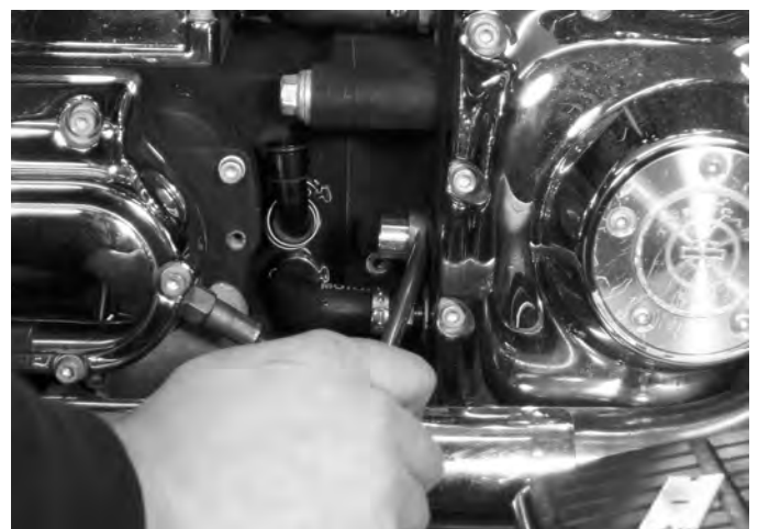
10. Install female fitting into engine block and slide springs onto hose.
